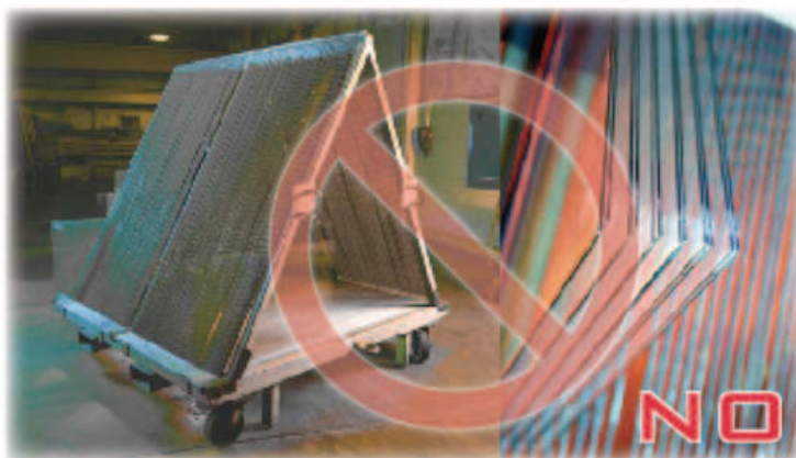
Figure 5. Harp Racks Are Not Recommended for Coated Products
