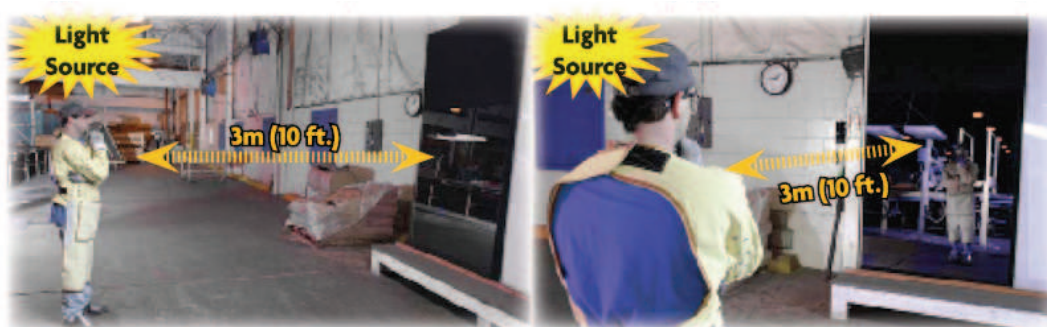
Figure 12. Visual Inspection of Reflection (Light Source Behind or Above Inspector)
