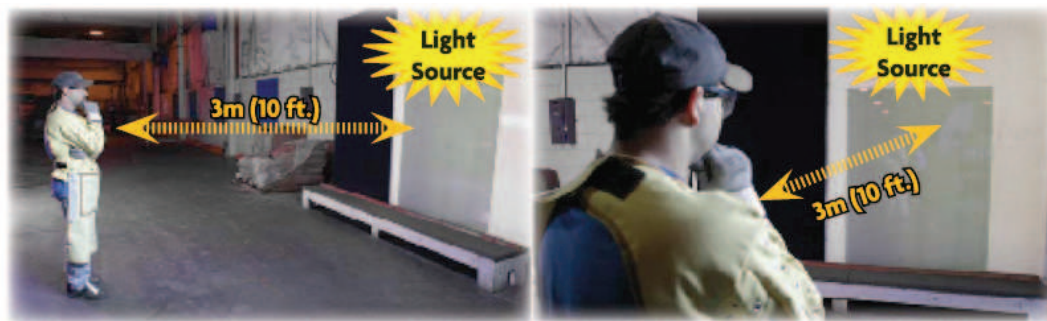
Figure 11. Visual Inspection of Transmission (Light Source Behind Glass)
