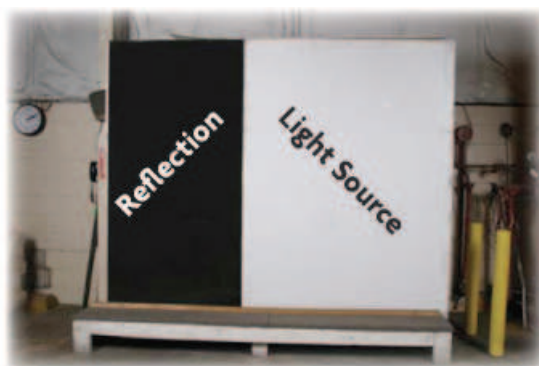
Figure 10. A Common Artificial Light Source and Reflection Setup
